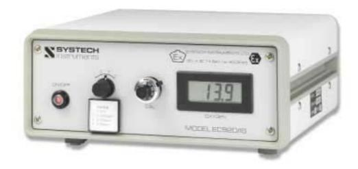
The EC92DIS portable oxygen analyser will detect levels of oxygen as low as 0.1ppm, up to high percent levels and can be used on most industrial gases and atmospheres. There is no need for routine maintenance of the fuel cell, and the instrument may be easily calibrated, using ambient air or standard calibration samples.
