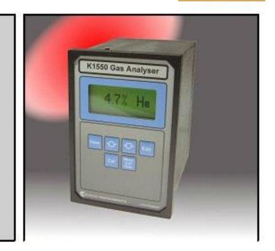
The Hitech K1550 accurately measures the changes of one constituent in binary or pseudobinary gas mixtures (ie, mixtures in which only one constituent changes). Examples include hydrogen, carbon dioxide, argon, helium and various halogenated hydrocarbons such as the Freons. Almost any single constituent of a gas mixture can be measured providing its thermal conductivity differs from that of the other components. Ranges from high ppm to 100% are possible depending on the gas being measured.
