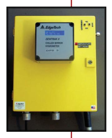
Model DPS3 is a heated dew point hygrometer that can measure dew points up to 95°C (203°F) and as low as -35°C (-31°F). This integrated system includes a microprocessor based electronics, a chilled mirror dew point sensor, a sample flow meter/valve, a 3 foot heated sample line, assorted tubing and fittings; all contained in a heated, temperature controlled NEMA-4 enclosure.
